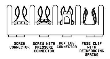
FIGURE 2. Wire termination configuration.
