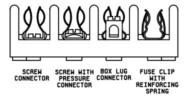
FIGURE 2. Wire termination configuration.
