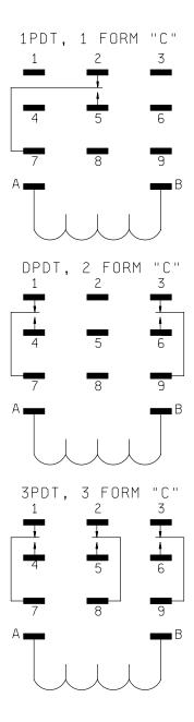
FIGURE 2. Circuit diagrams (terminal view).
