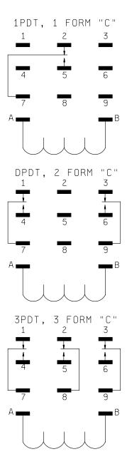
FIGURE 2. Circuit diagrams (terminal view).
