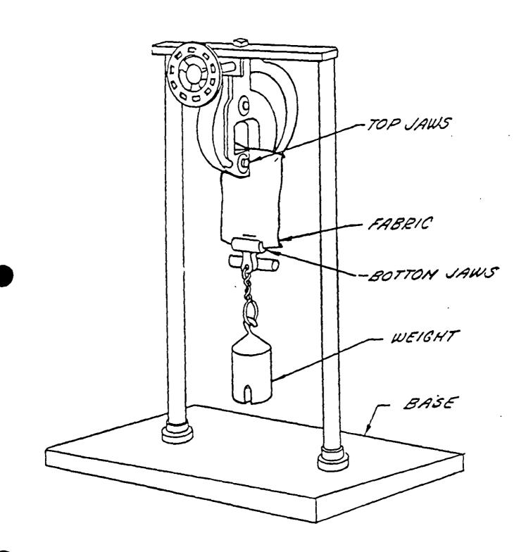
FIGURE 2. Fabric Stretch Apparatus
