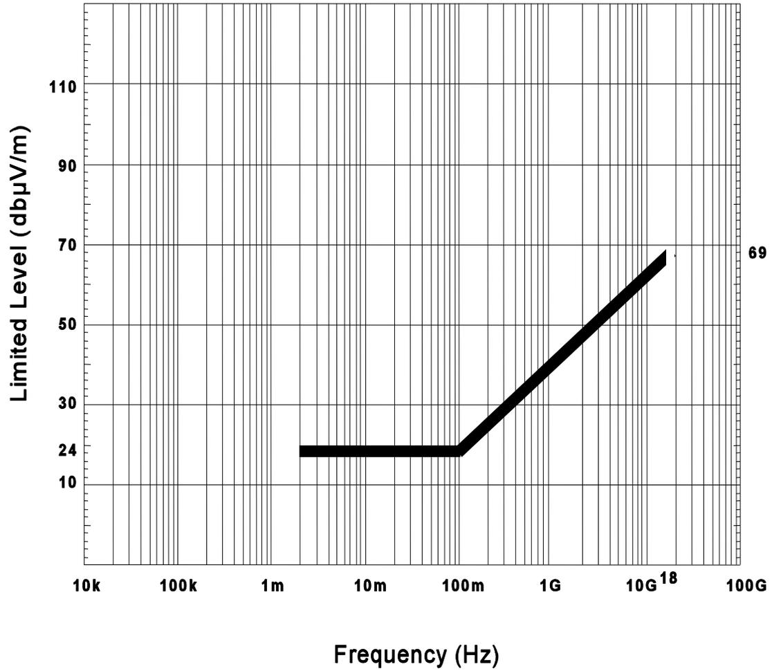
Figure 4. Radiated emission limit .
