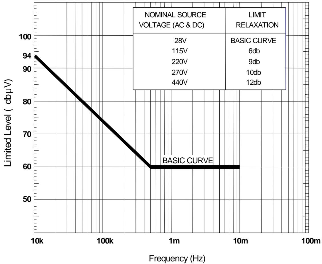
Figure 2. Conducted emissions limit
