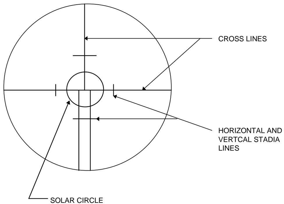
Figure 1. Reticle pattern for theodolite.
