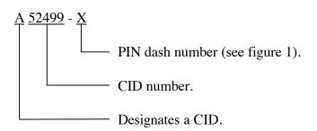
5.4 <u>Cross-reference data</u>. Leads conforming to this CID are interchangeable/substitutable with leads conforming to MS35915B. The CID dash numbers and the MS dash numbers are the same.
