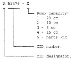
d. <u>Cross-reference data</u>. Pumps conforming to this CID are substitutable with pumps conforming to MIL-P-3306E, dated 17 August 1987, and MS51084C, dated 17 January 1986. PIN number to former part numbers are as follows:
