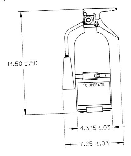
NOTE : Dimensions are in <sup>inches</sup>. FIGURE 1. Complete unit <sup>overall</sup> dimensions.
