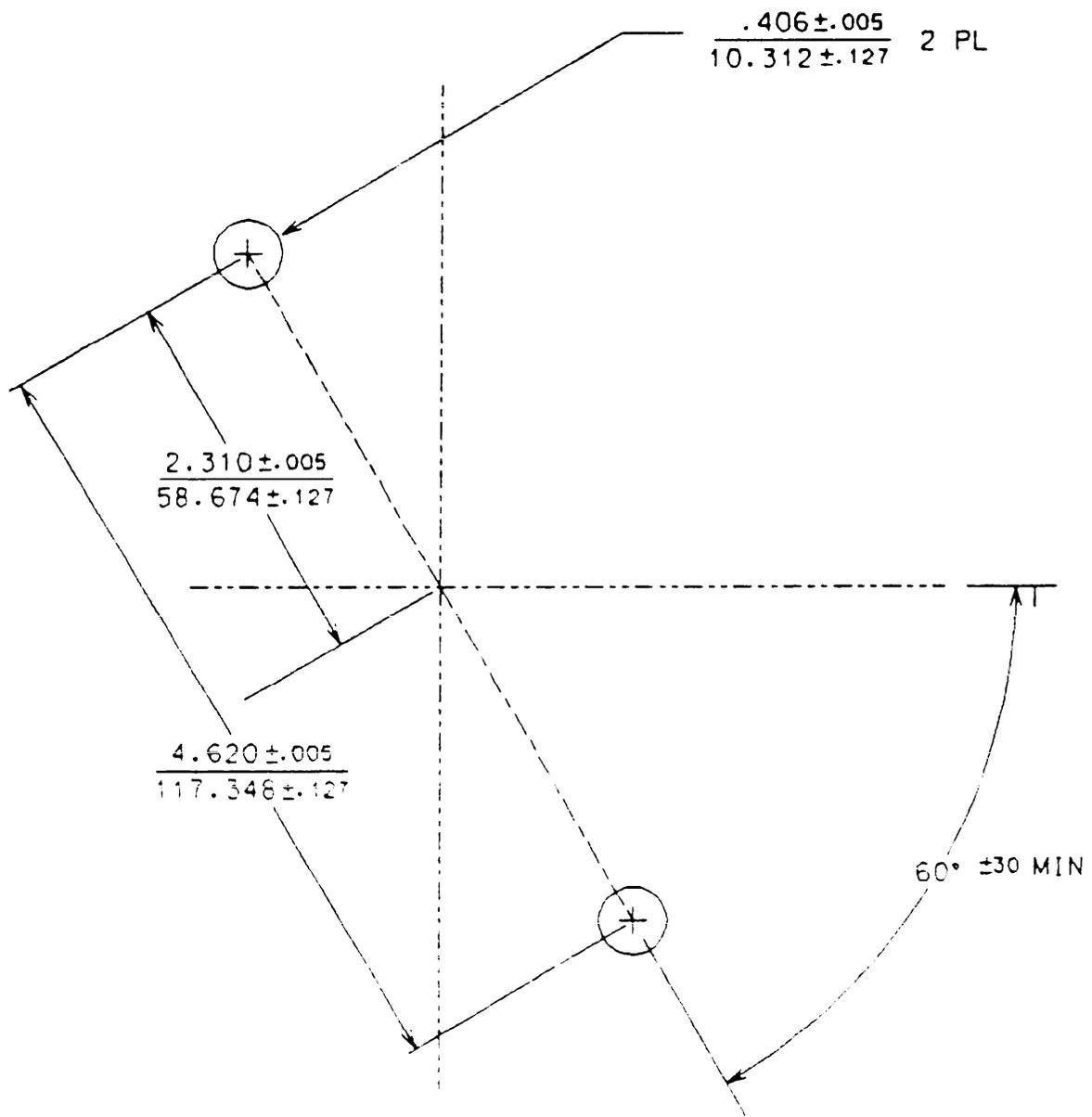
FIGURE 1. Mounting dimensions.
