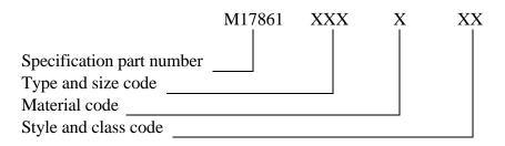
7.1.1 Type and size to code identifier. The type and size of the pump unit is identified by a threedigit identifier as shown in table V. The first number identifies the type; the second and third numbers identify the size.
