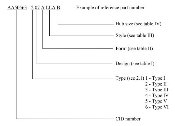
AA50563-2 07 A LLA B identifies a rectangular base general purpose conduit outlet box; threaded hub connection for rigid conduit, shallow depth; single gang; one hub in one end and one hub in the back; 3/4-inch hub size.
