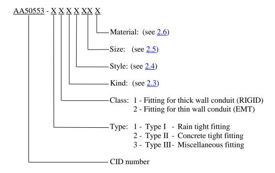
Example of reference part number: AA50553 - 11D203Z identifies a type I rain tight fitting, thick wall conduit, threaded 45 degree electrical connector box, insulated throat, 1-inch, made of zinc alloy.
