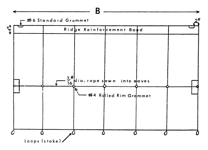
Number of seams, grommets, and stake down loops shown in figures 1&2 does not represent actual number that may be needed.
