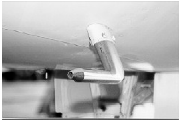
Figure 10-5. Typical Pitot tube installation, underside fuselage w/o integral static port.
