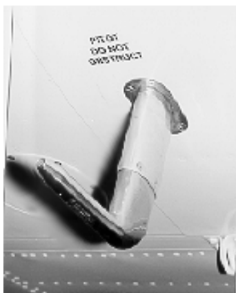
Figure 10-6. Typical Pitot tube installation, underside wing w/o integral static port.
