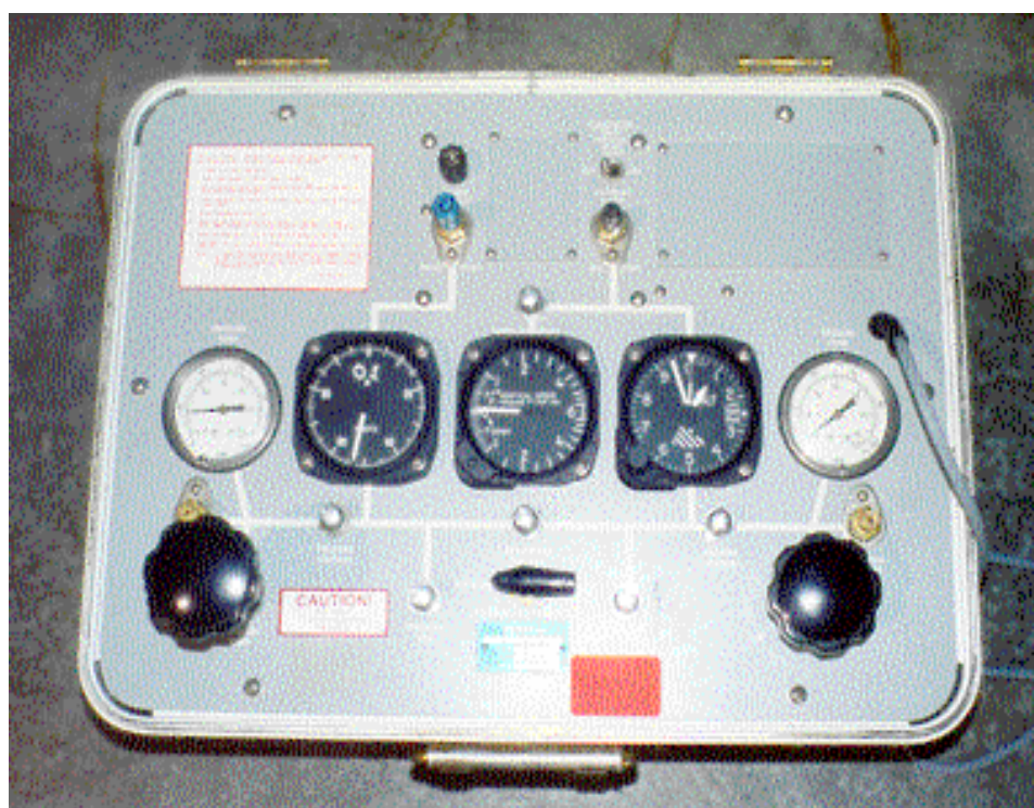
Figure 7-5. Barfield Pitot-static ramp test set.
