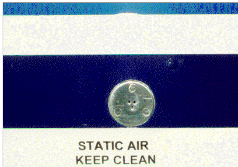
Figure 10-7. Standard static port installation on side of fuselage.
