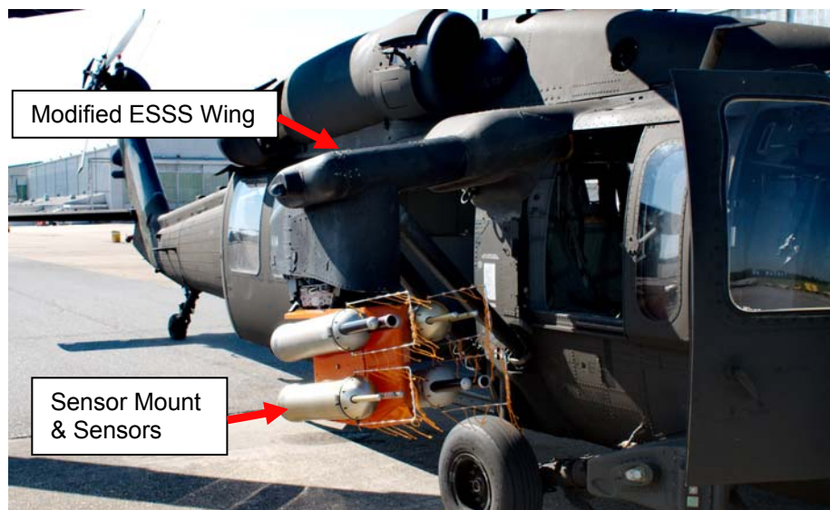
Figure 3. UH-60M Configured for Icing Tests
