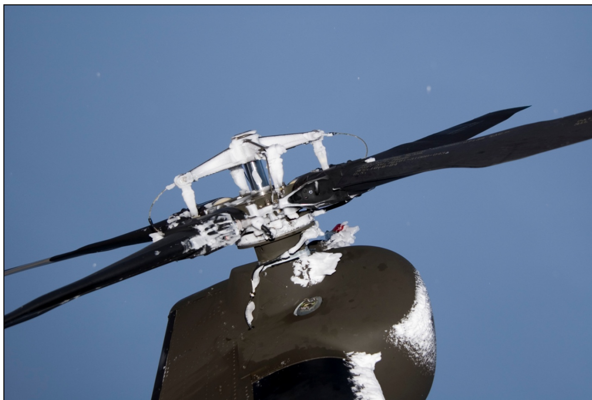
Figure XX. Ice Accretion on Tail Rotor Hub
