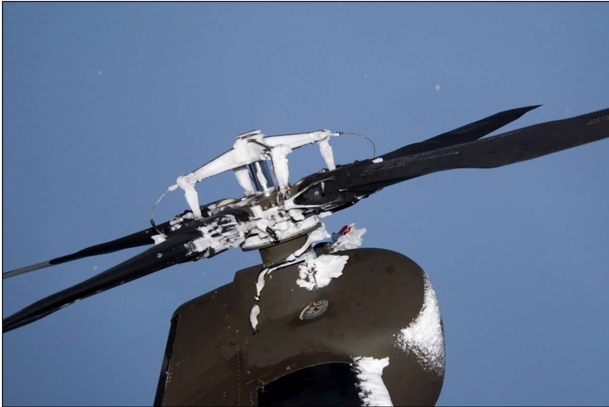
Figure XX. Ice Accretion on Tail Rotor Hub
