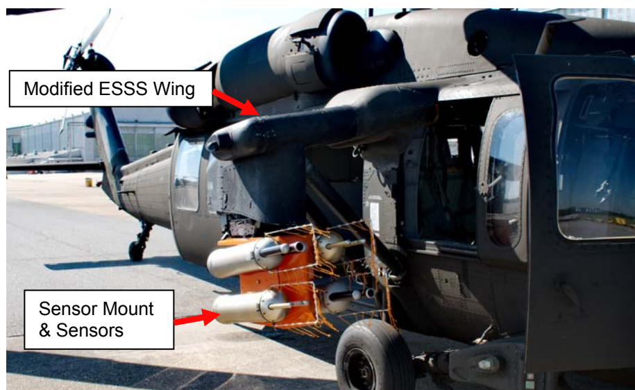
Figure 3. UH-60M Configured for Icing Tests
