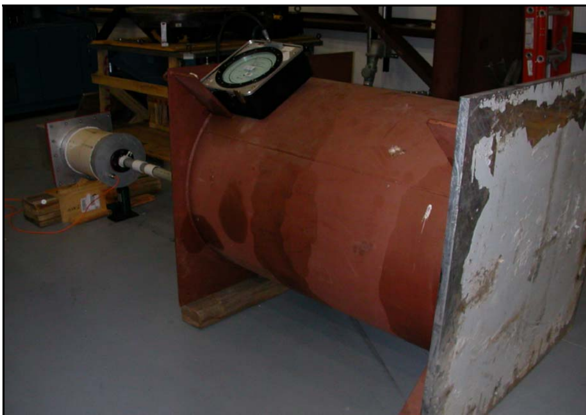
Figure 1. Typical Rapid Decompression Test Setup
