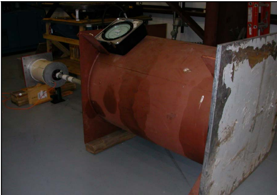
Figure 1. Typical Rapid Decompression Test Setup
