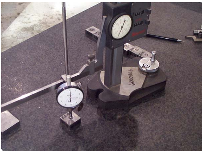
Figure 3. Dent Block Depth Measuring Device - Dial Indicators
