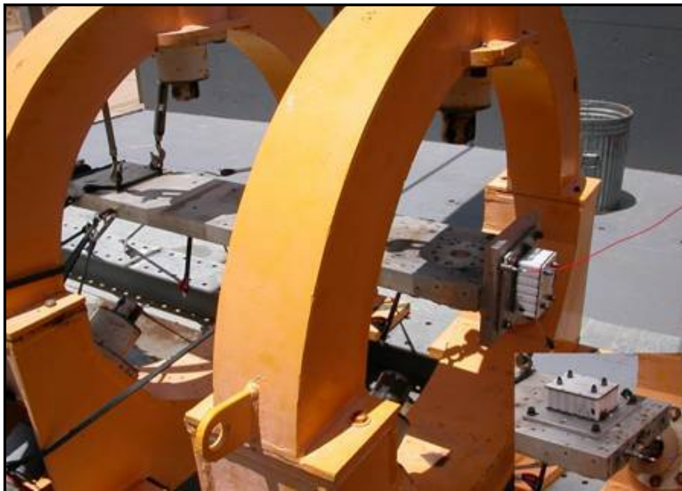
Figure 2. Typical Resonant Beam Test Fixture Suspended With Test Item Attached (2 orientations)
