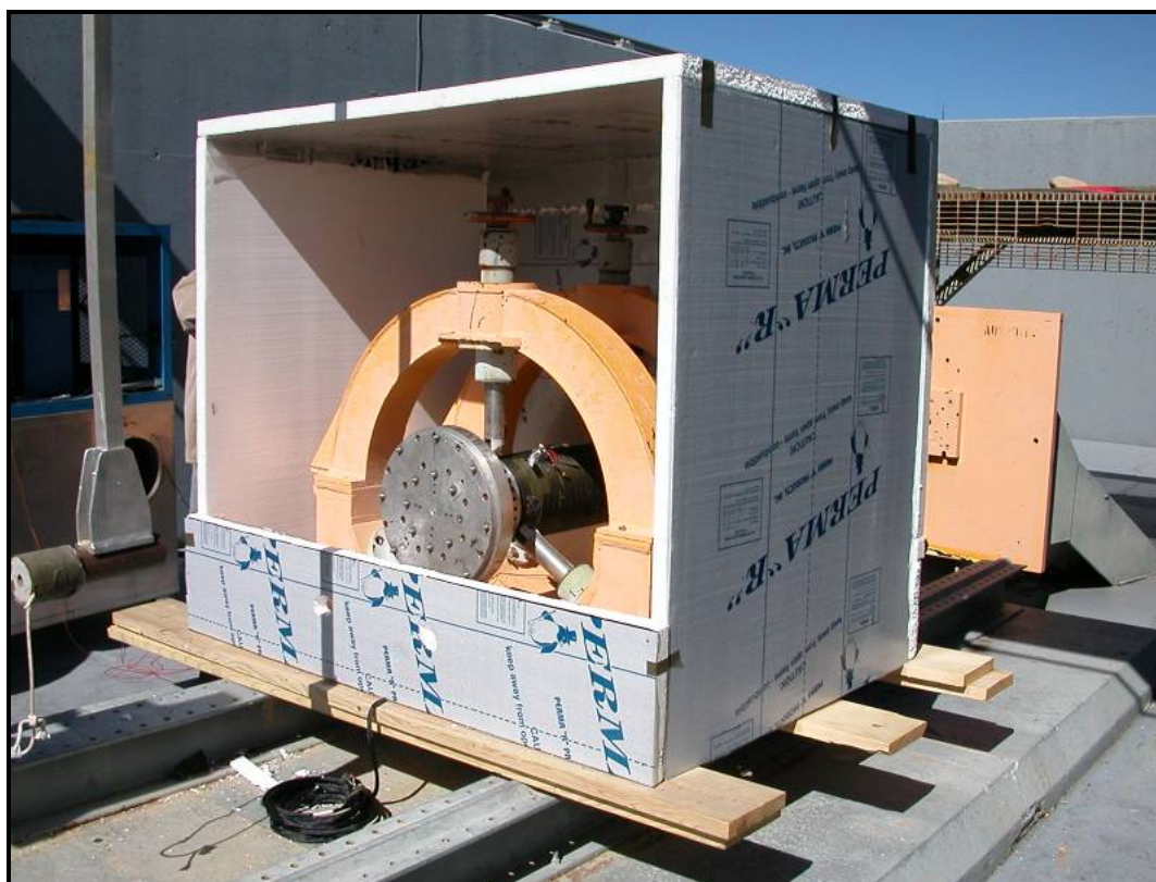
Figure 1. Open Temperature Conditioning Shroud Encompassing Entire Pyroshock System
