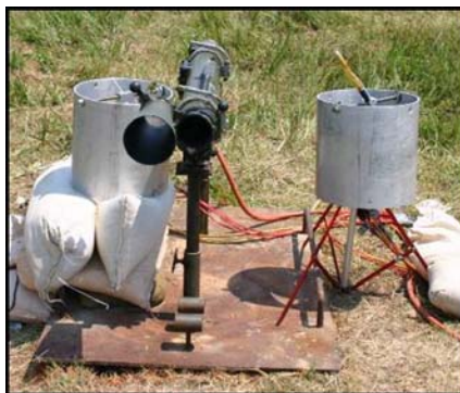
Figure 4. Example of Blast Test Device Cut Down in Height to Accommodate a Specific Weapon Firing Configuration.
