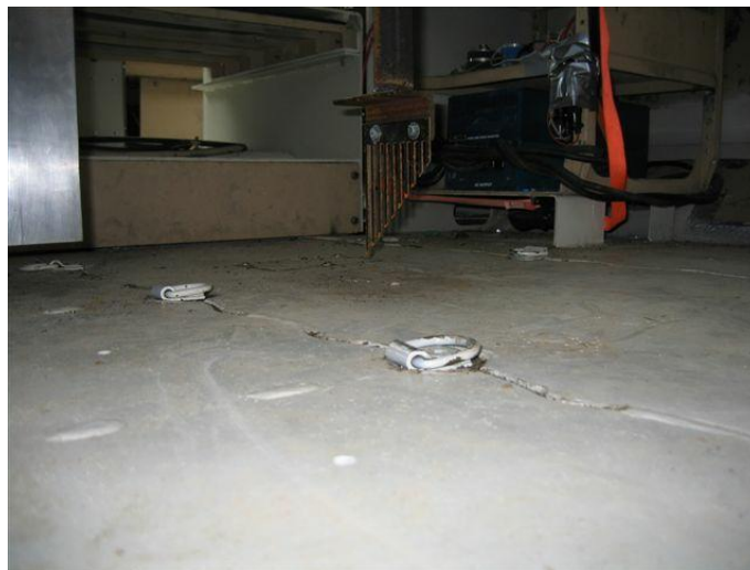
Figure 13. Comb Gage suspended from a vehicle ceiling, used for measuring floor displacement during a ballistic event.
