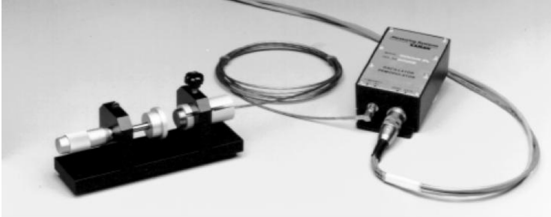
Figure 10. Typical Eddy Current setup for the Kaman Model KD-2300. The sensor itself is mounted in the fixture to the left with cabling leading to an electronics module shown on right.
