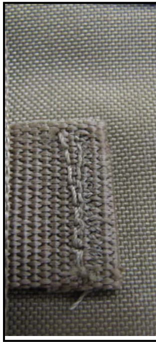
Figure E-3. Bartack not constructed properly.
