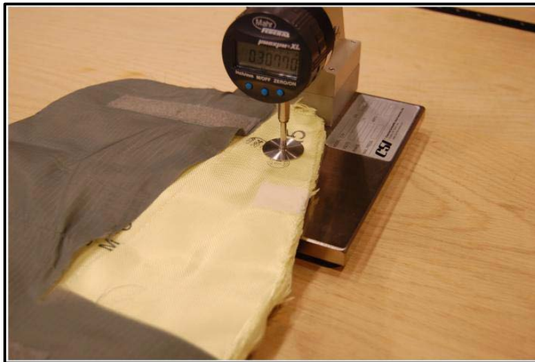
Figure F-3. Ballistic filler thickness.
