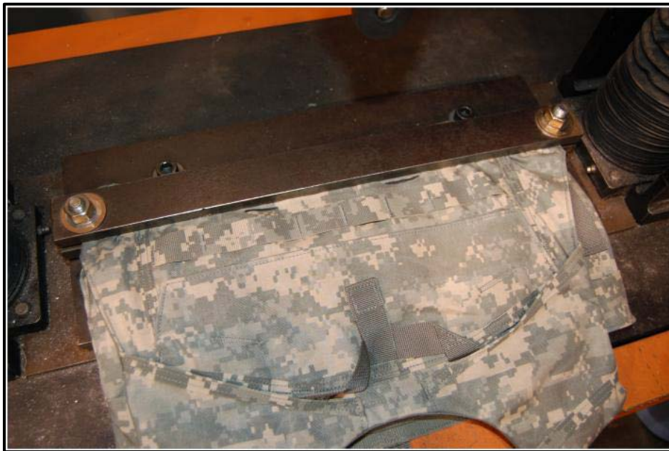
Figure F-11. Carrier set up on second bar of test fixture.
