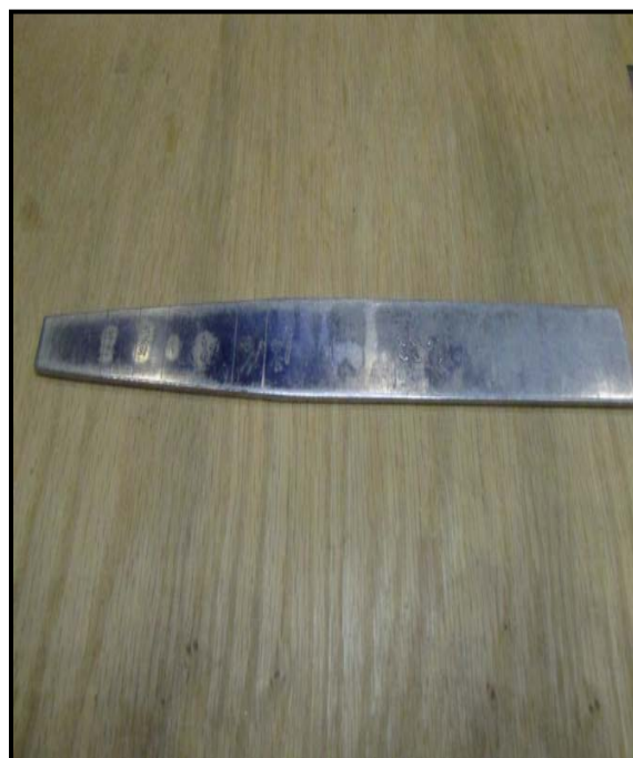
Figure D-10. ATC buttonhole measuring device.
