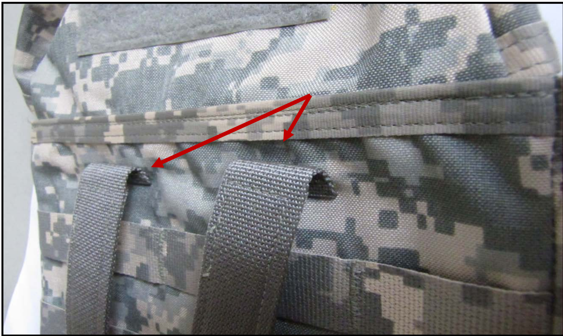
Figure E-7. Components joined together incorrectly.
