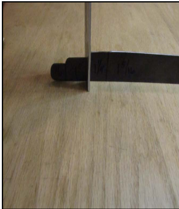
Figure D-8. ATC loop height measuring device.
