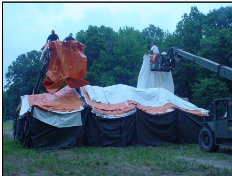
Figure 10. Snow load test of framed tent
