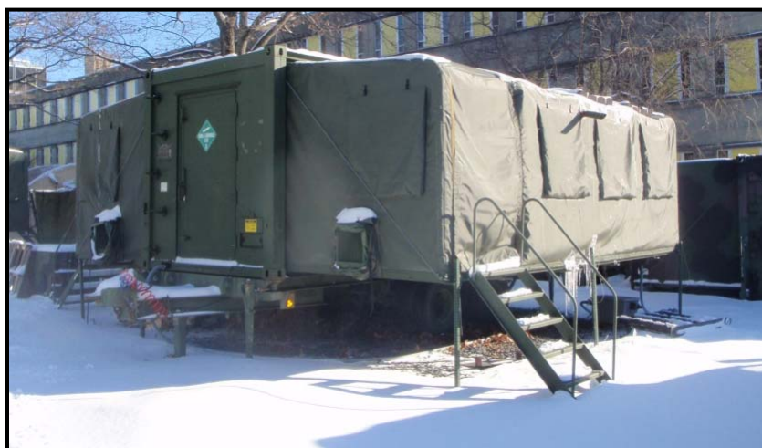
Figure 6. Hybrid shelter with rigid walls and soft fold-down walls.
