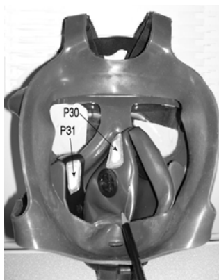
Figure E.49. Inside View of M40 Mask, P30 and P31 PAD Locations.
