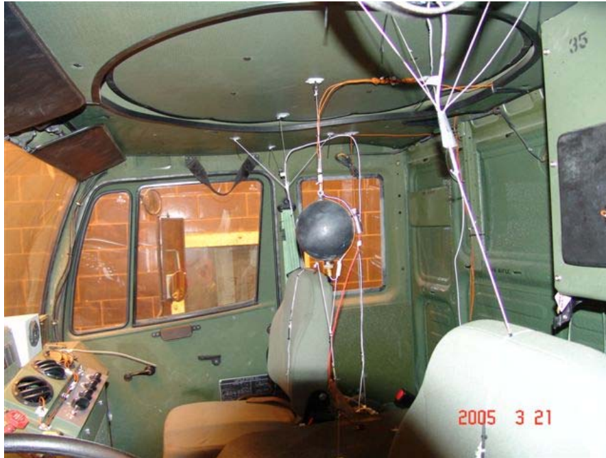
Figure 1. Instrumentation installed in cab for Family of Medium Tactical Vehicles (FMTV)
