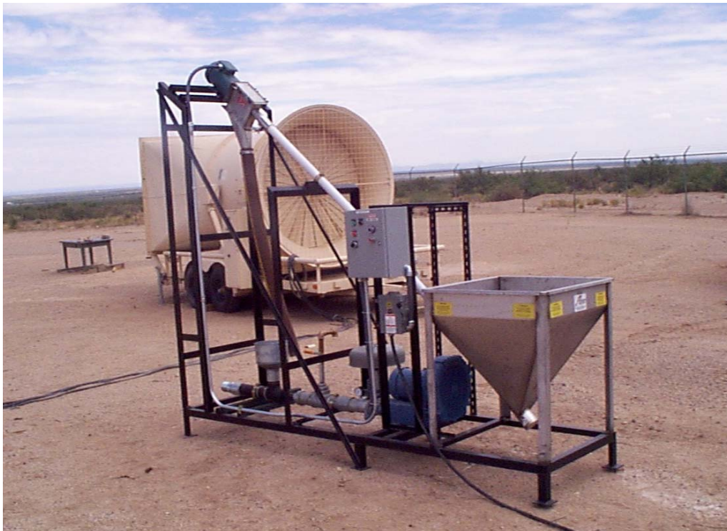
Figure 1. Typical Sand and Dust Injection System with 200 HP Wind Generator in Background
