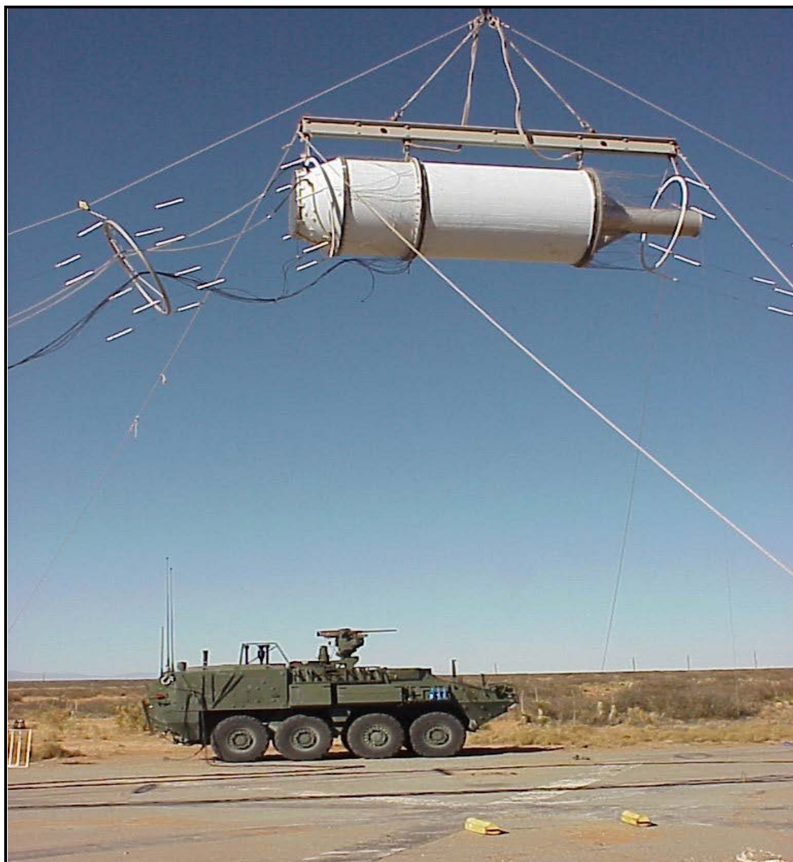
Figure C-1. Generic missile launcher HEMP test setup.
