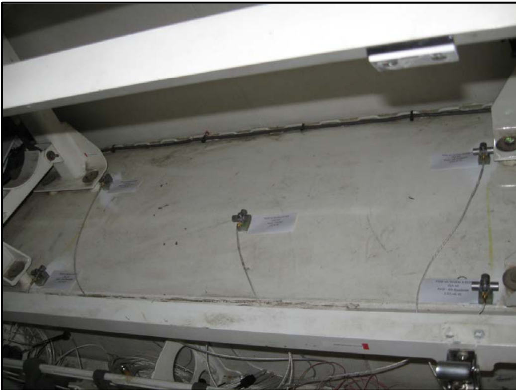
Figure 4. Transducer placement (input to missile rack).
