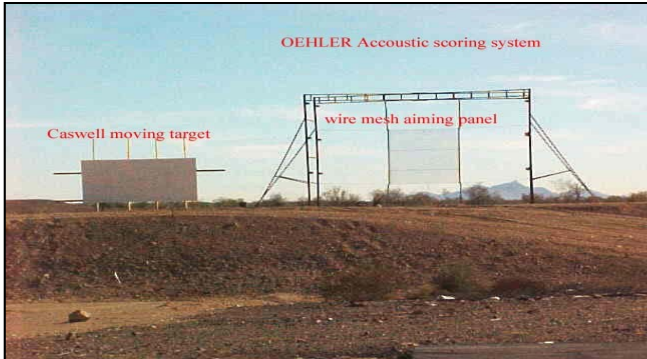
Figure 172. Remote controlled rail-mounted carriers equipped with pop-up targets and an Oehler acoustic scoring system target.
