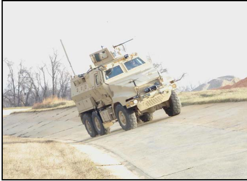
Figure 42. Vehicle negotiating the 20-percent side slope.
