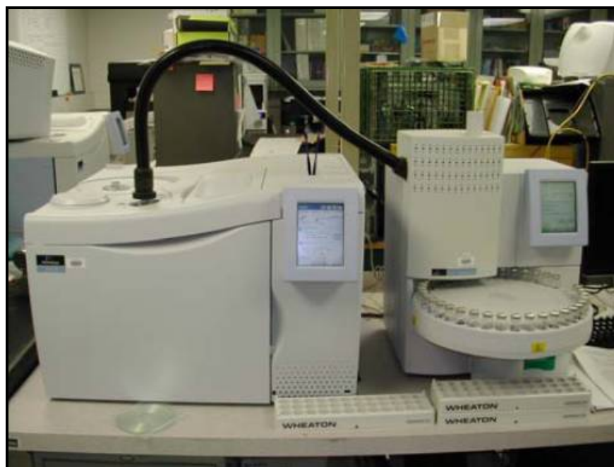
Figure 185. Gas chromatograph with turbomatrix heads pace sampler used to measure diesel fuel dilution.
