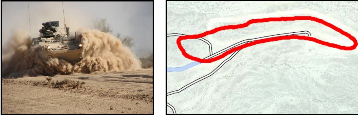
Figure 130. Vehicle performing non-convoy dust testing on Kofa Dust Course (left) and map of Kofa Dust Course (right).
