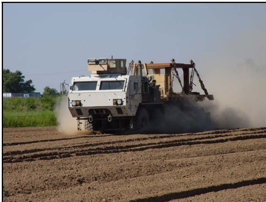
Figure 29. Crossing velocity test in the hog wallow.
