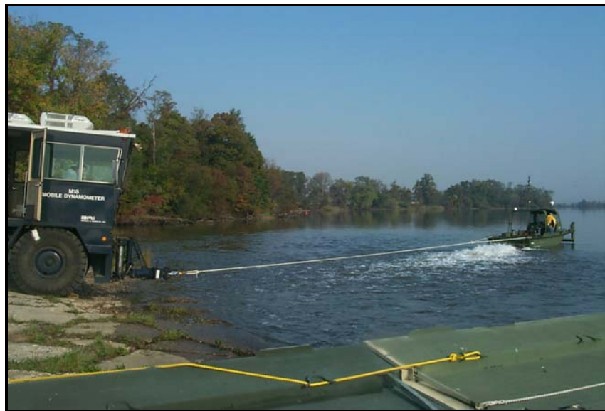
Figure 35. Bollard pull using mobile field dynamometer.
