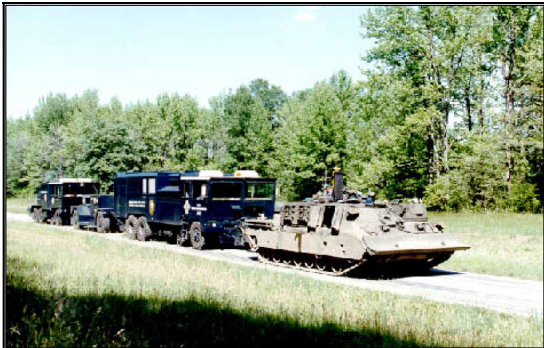
Figure 12. Drawbar pull test conducted on Dynamometer Course.
