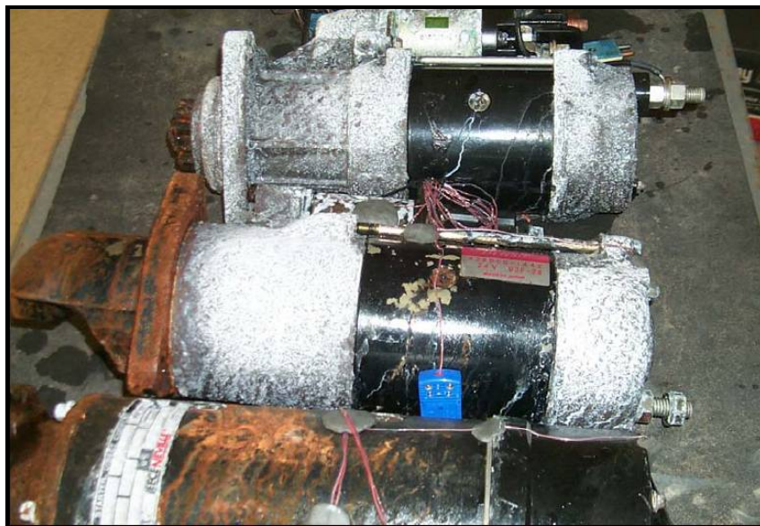
Figure 181. Test item after climatic salt fog testing.
