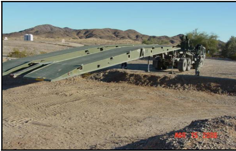
Figure 161. Bridging device test ditch.
