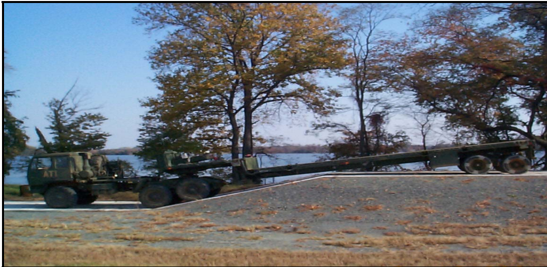
Figure 46. Vehicle on 15-degree simulated loading ramp.
