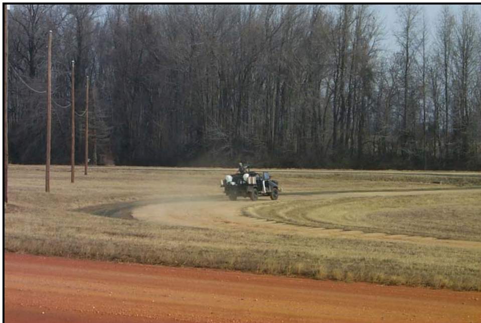
Figure 51. Vehicle testing on the 2- to 4-Inch Radial Washboard Course.
