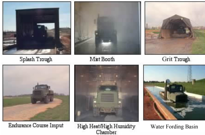
Figure 27. Accelerated Corrosion Complex.
