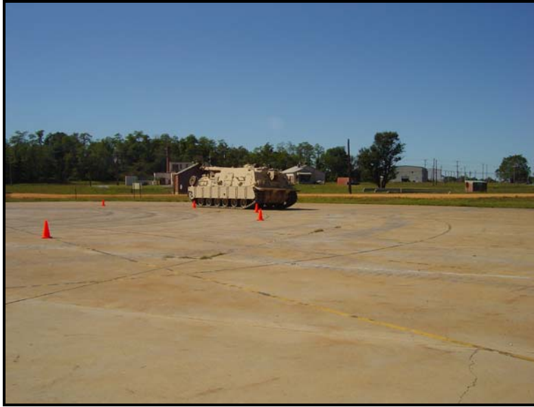
Figure 62. Measurement of vehicle turning diameter on the Munson Turning Circle.
