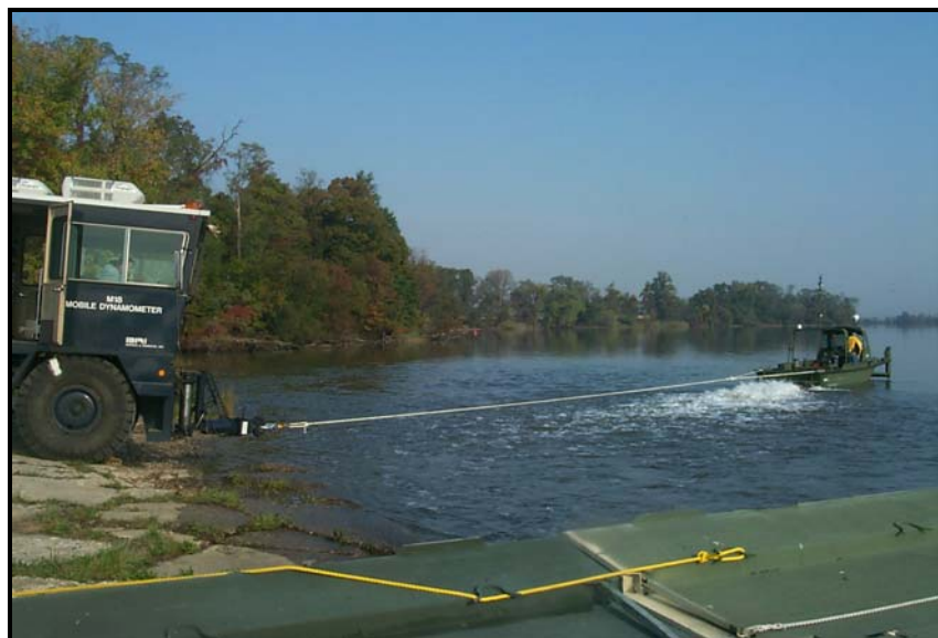
Figure 35. Bollard pull using mobile field dynamometer.
