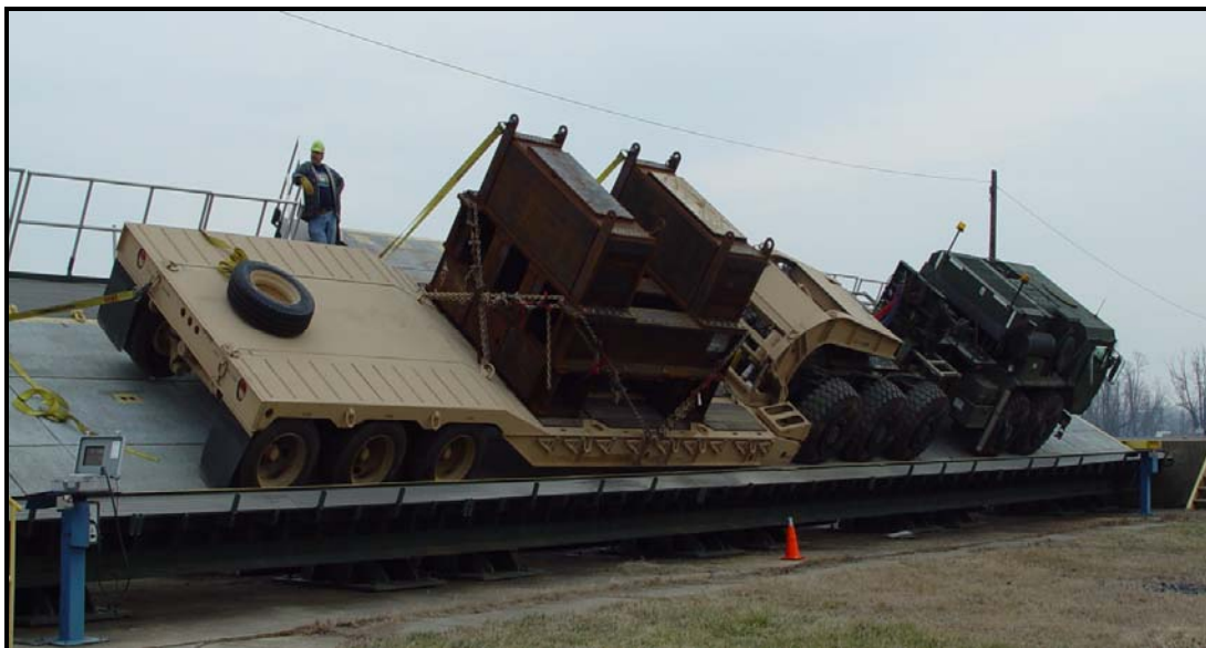
Figure 84. Tilt Table Facility.
