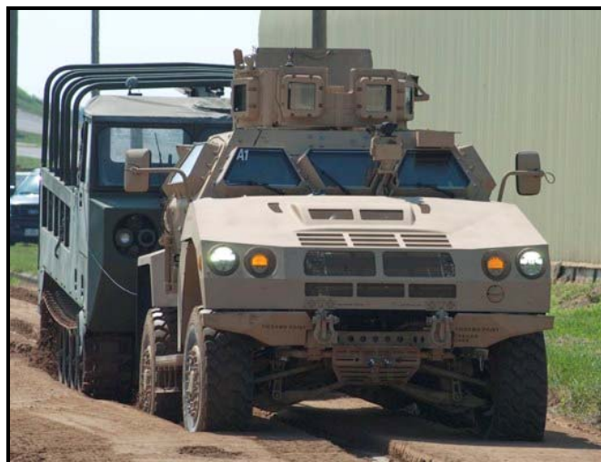
Figure 25. Drawbar pull testing in Sand Course.
