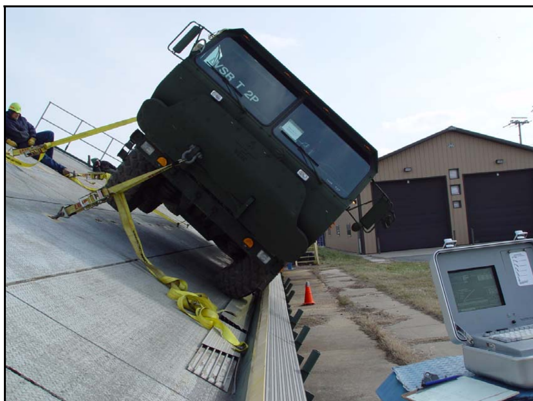
Figure 85. Tilt table testing to determine roll over threshold.
