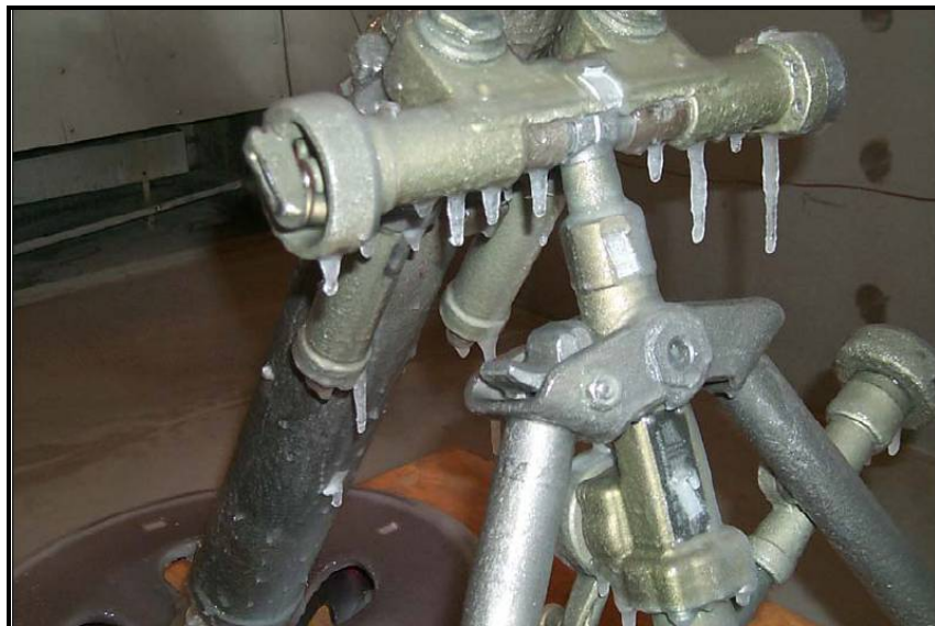
Figure 180. Test item after climatic icing test.
