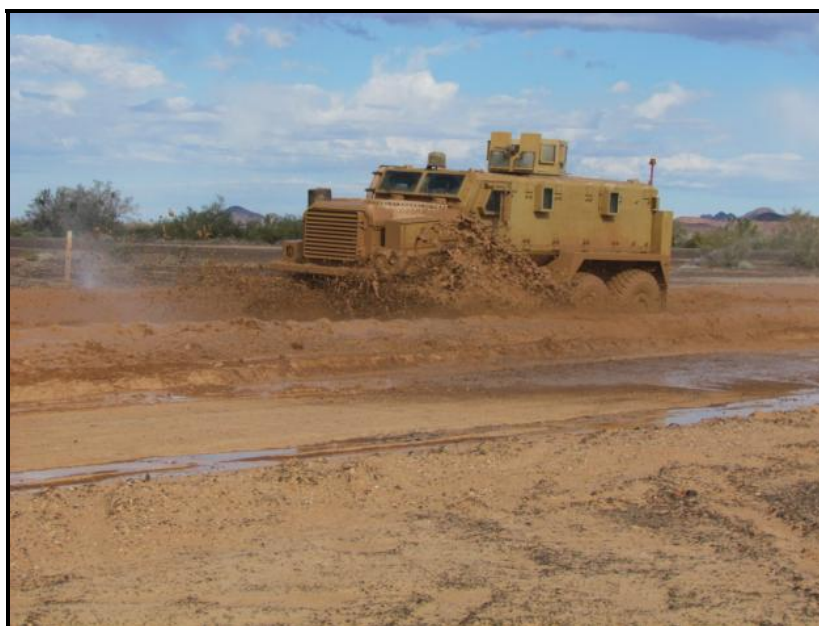
Figure 132. Vehicle operating on Dyno Mud.
