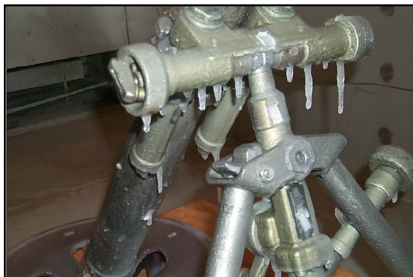
Figure 180. Test item after climatic icing test.
