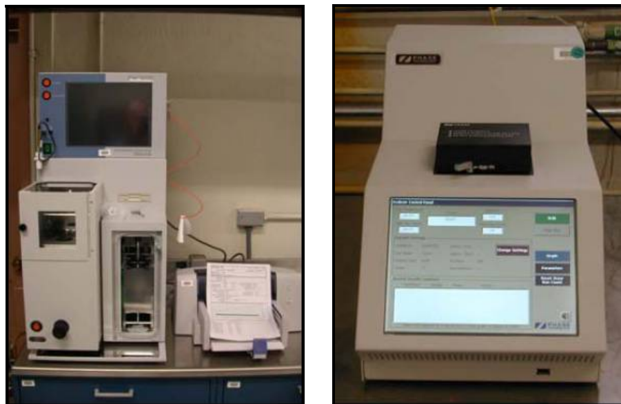
Figure 186. Automatic distillation unit used to measure fuel distillation (left) and automatic cloud and pour point used to measure low temperature characteristics (right).
