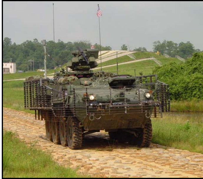
Figure 40. Durability testing using Imbedded Rock Course.
