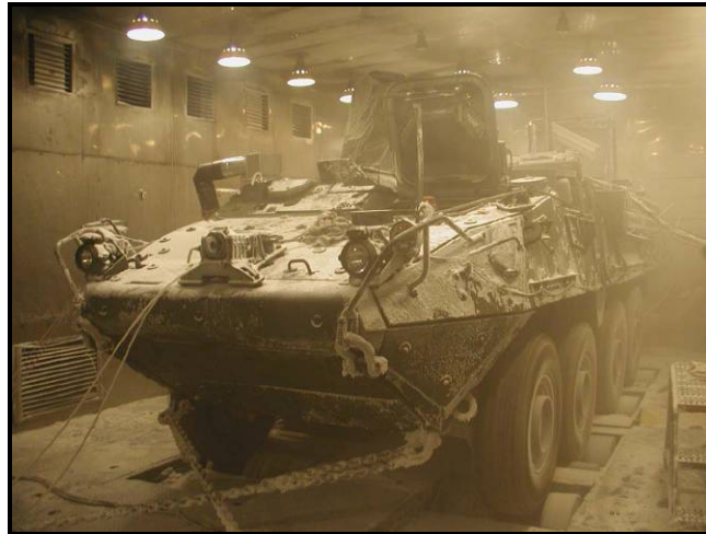
Figure 178. Test vehicle operating on the chassis dynamometer at -32 °C (-26 °F).
