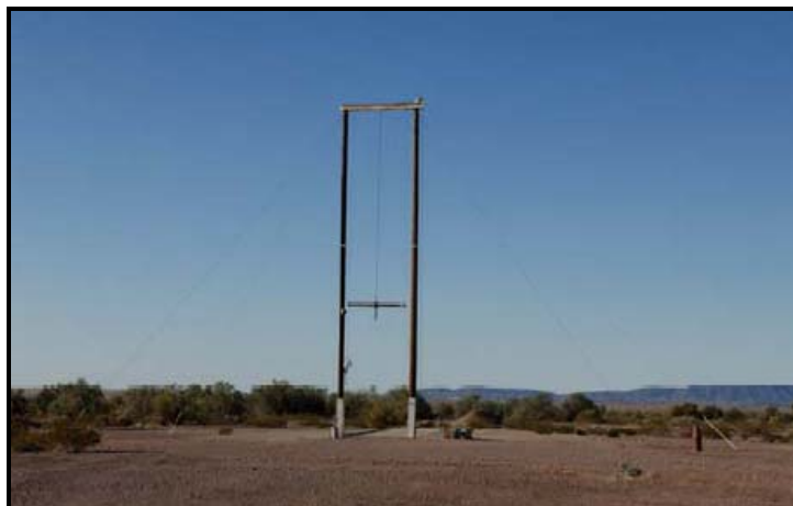
Figure 192. 12 Meter Drop Test facilities.
