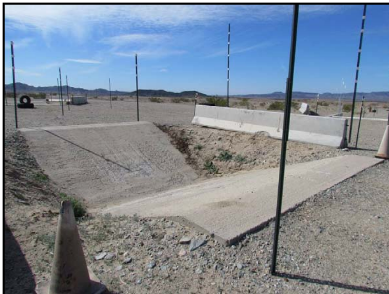
Figure 148. Direct approach V-ditch.
