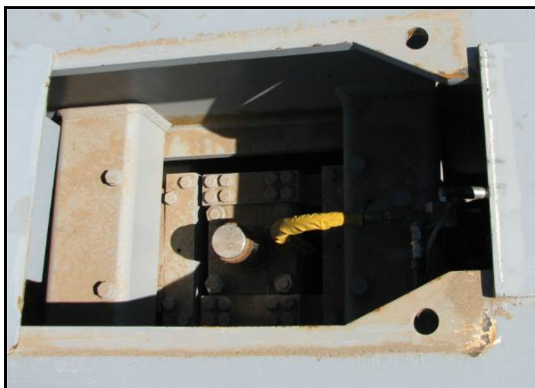
Figure 159. LTTF vertical hydraulic ram (located under the surface of the LTTF bed).
