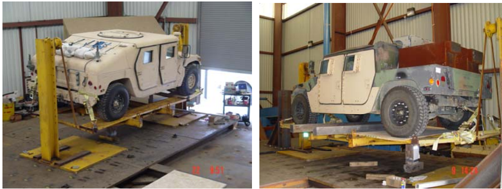
Figure 90. Vehicles subjected to inertia tensor and center of mass testing.
