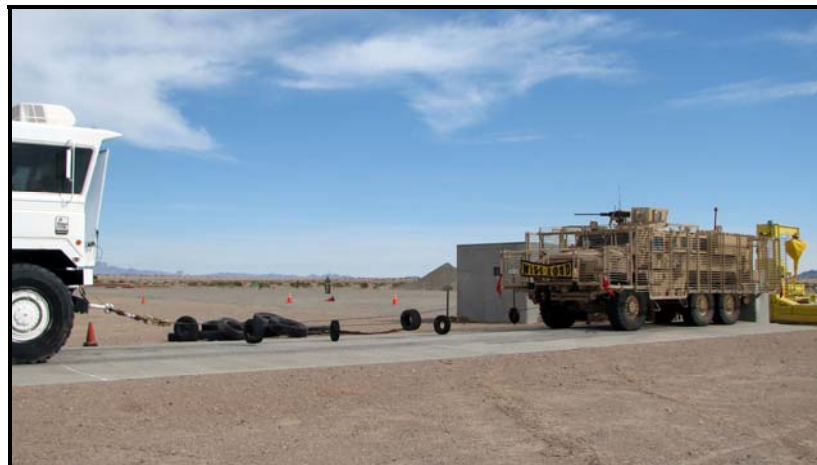
Figure 155. Vehicle undergoing winch testing.
