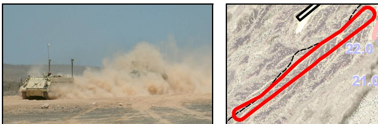
Figure 131. Vehicle performing convoy testing on Cibola Dust Course (left) and map of Cibola Dust Course (right).
