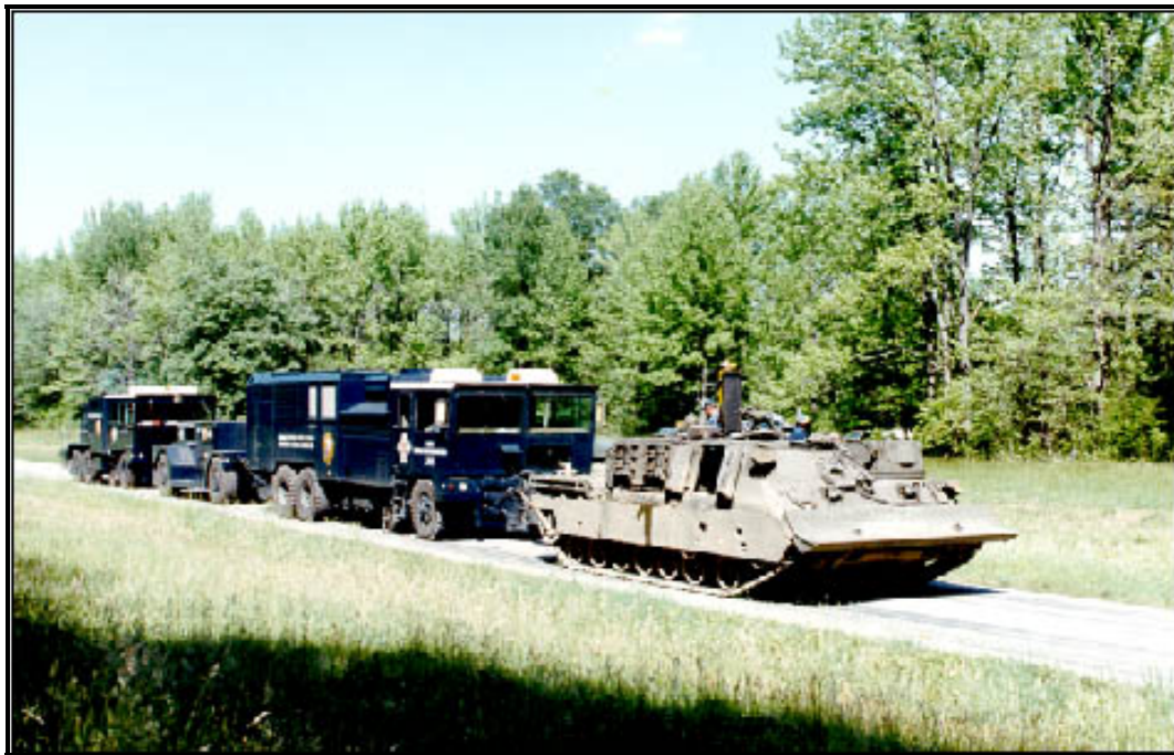
Figure 12. Drawbar pull test conducted on Dynamometer Course.
