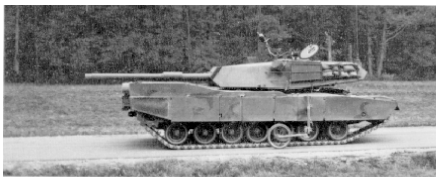
Figure 10. Fifth wheel attached to M-1 for brake test.
