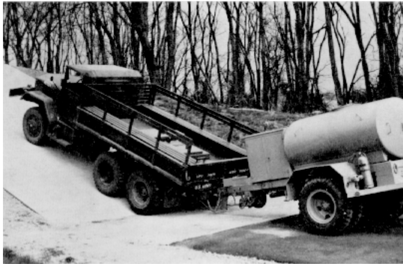
Figure 40. Vehicle on simulated loading ramp.
