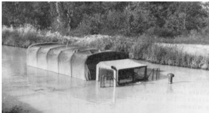
Figure 70. Vehicle in deep water fording facility.
