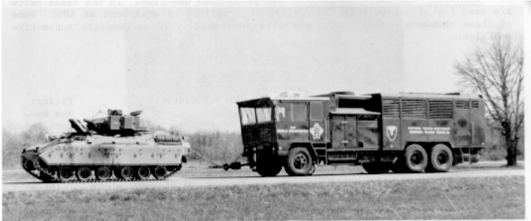
Figure 5. M-2 Infantry Fighting Vehicle undergoing drawbar pull test.
