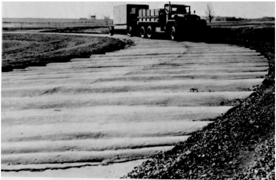
Figure 44. Radial washboard course.
