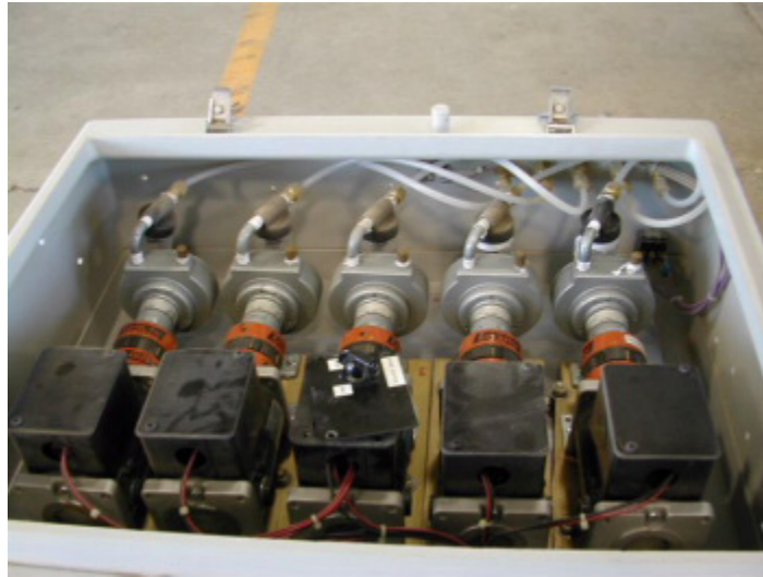
Figure D-4. Vacuum Pumps.
