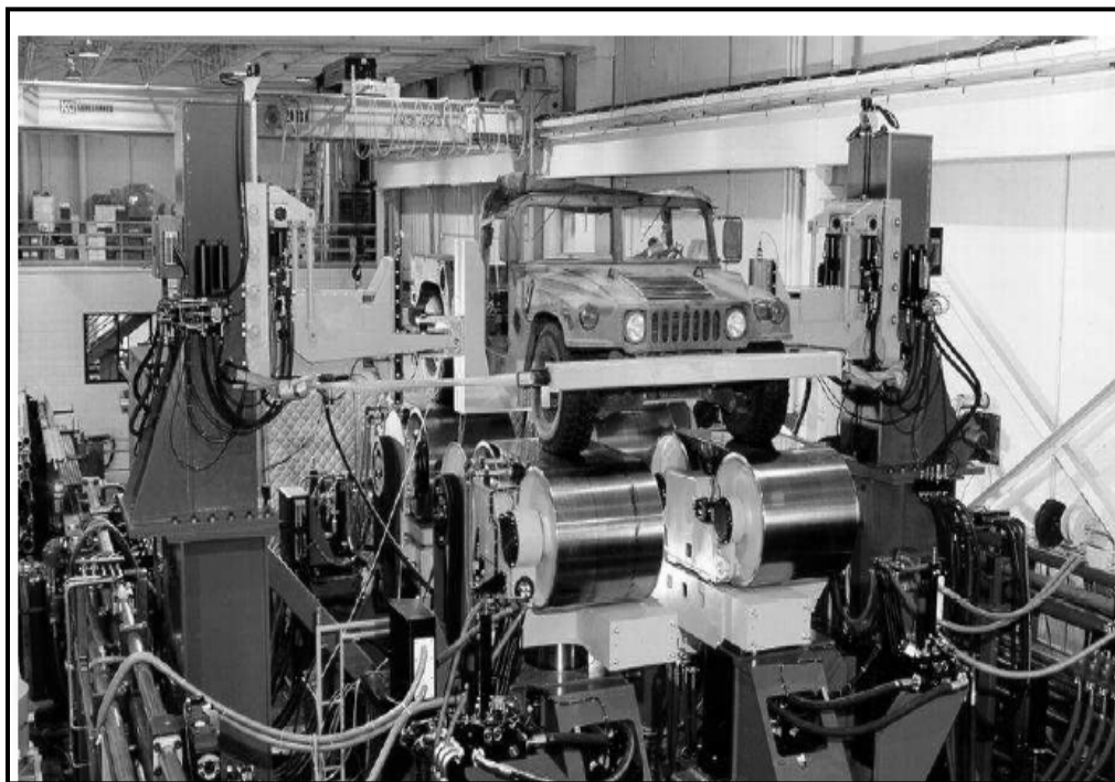
Figure 6. RWS configured for 2-axle testing.
