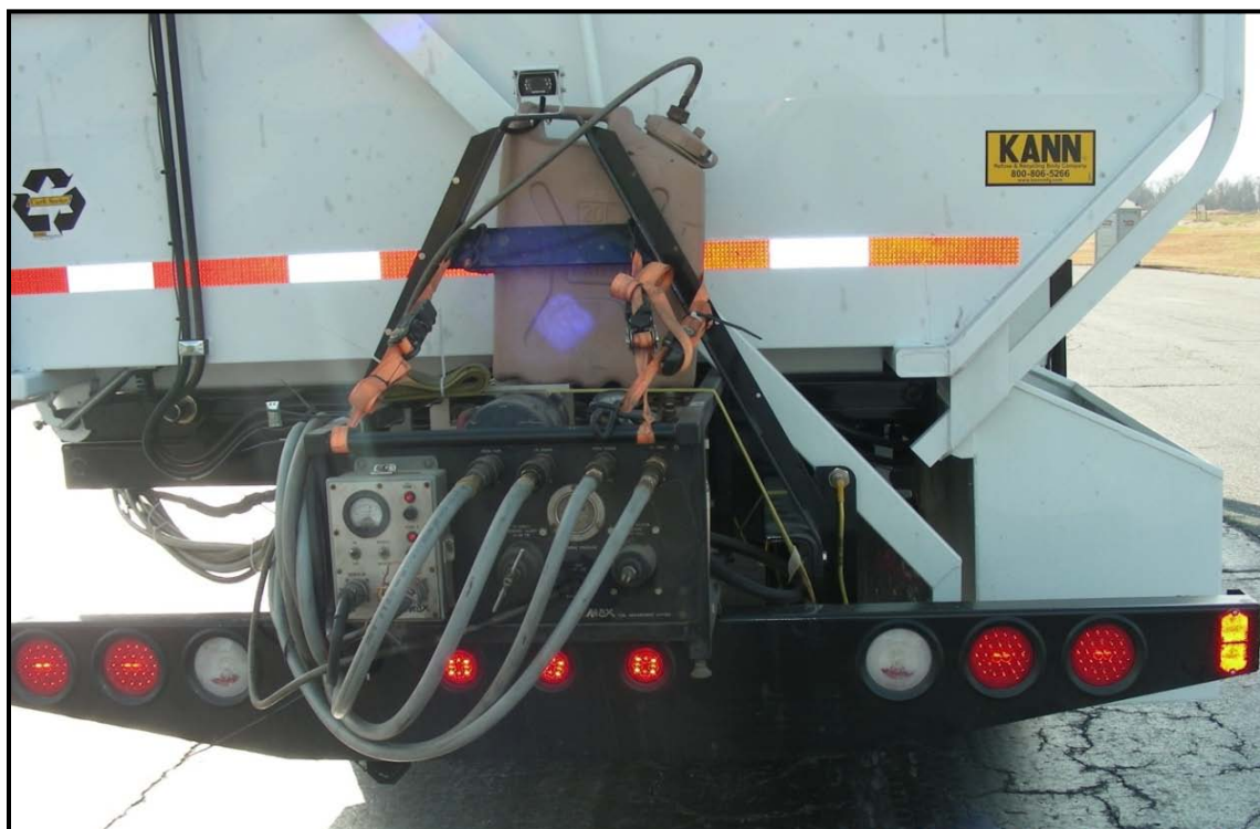
Figure 8. Model 910 Fuel Flow Measurement System installed on Hybrid Refuse Truck
