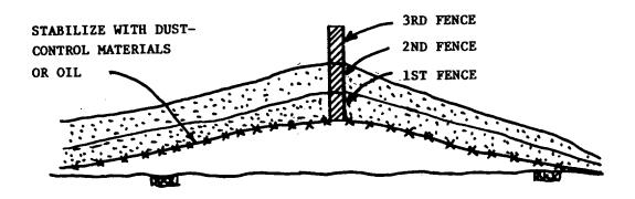
Figure B-3. Cross section of dune showing initial and subsequent fences.
