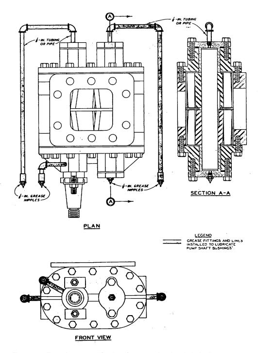
Figure 5-1. Typical pump modifications for conventional asphalt distributor.
