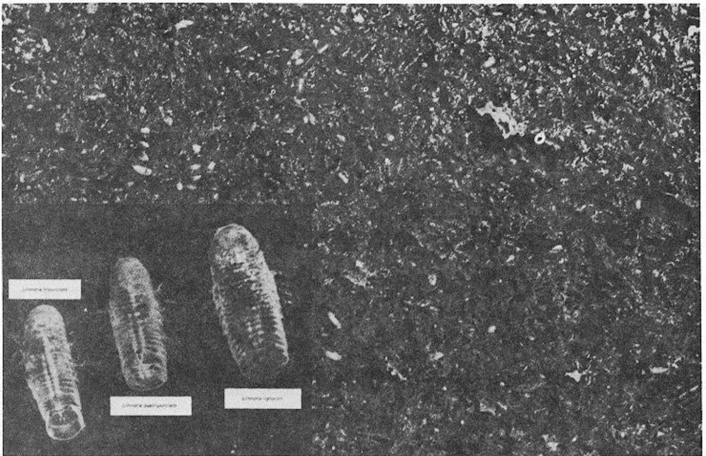
Figure 2-4. Surface of creosoted piling infested with Limnoria . Inset shows the three types of Limnoria .
