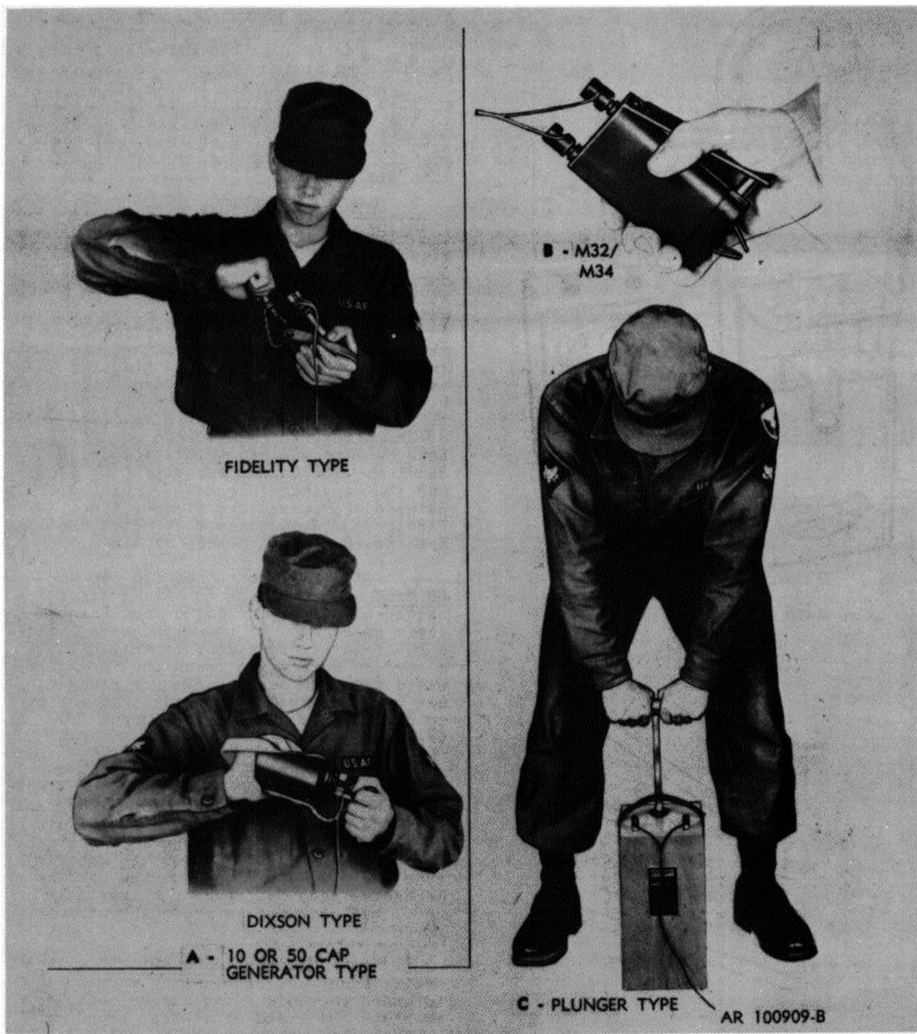
Figure 4-20. Actuating blasting machines.
