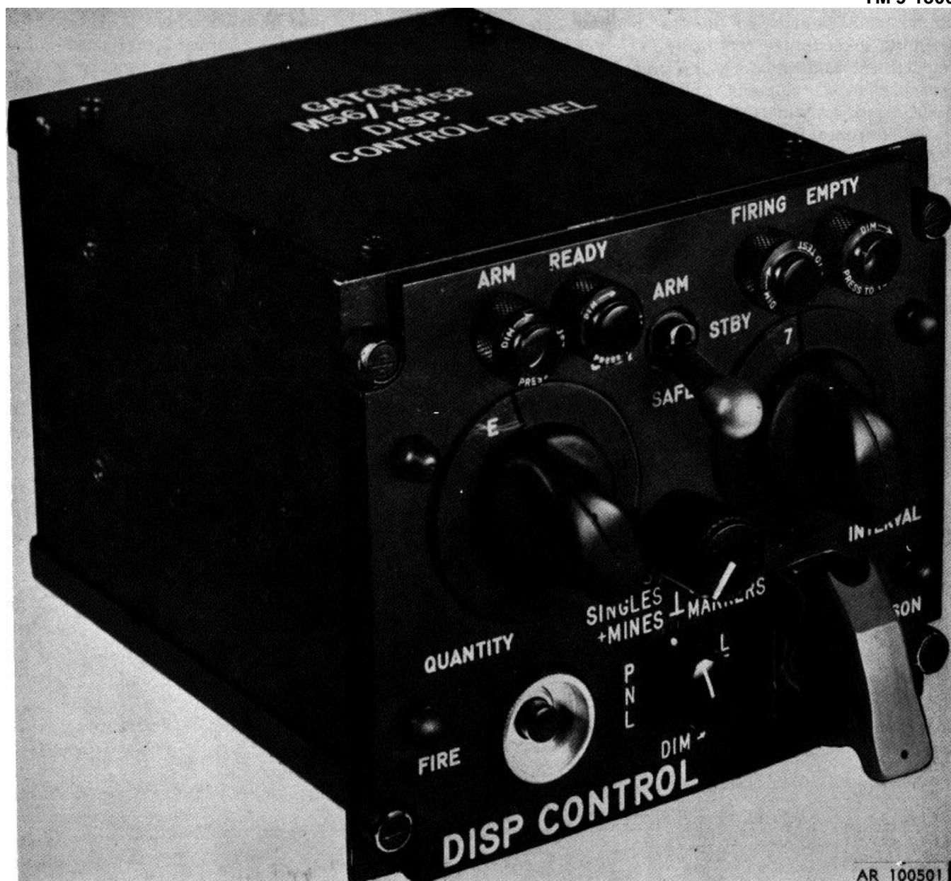
Figure 11-7. Mine dispersing subsystem, M56 dispenser (DISP) control panel
