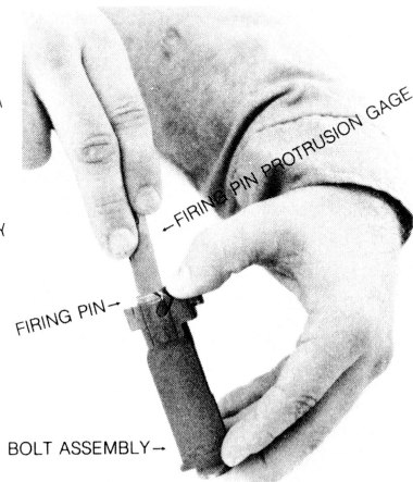
Figure 47. Gaging firing pin protrusion.
