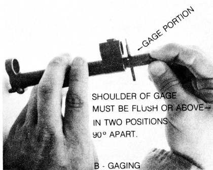
Figure 48. Reaming and gaging front interior of gas cylinder.
