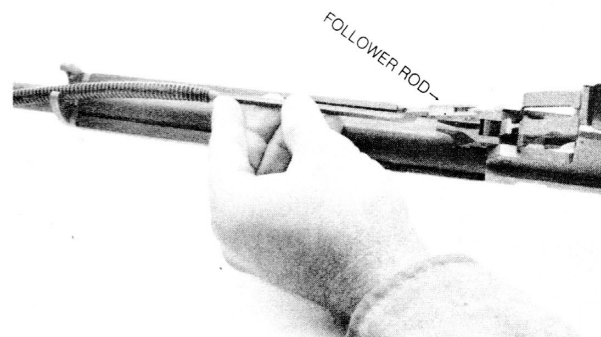
Figure 24. Removal / installation of operating rod assembly.
