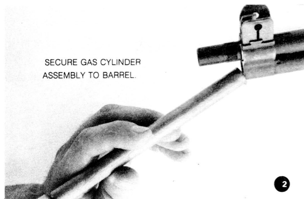
Figure 23. Disassembly / assembly of gas cylinder group (2 of 2).
