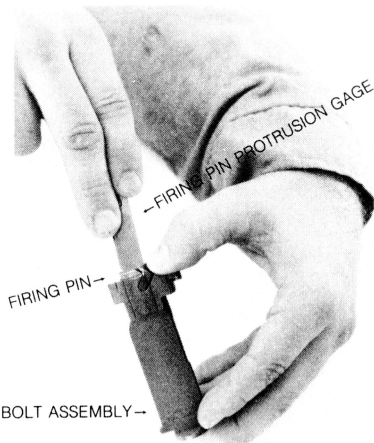
Figure 47. Gaging firing pin protrusion.
