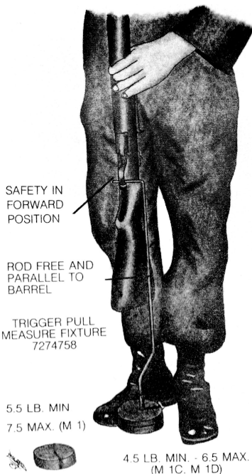
Figure 52. Checking trigger pull.
