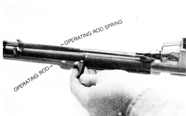
Figure 24. Removal / installation of operating rod assembly.
