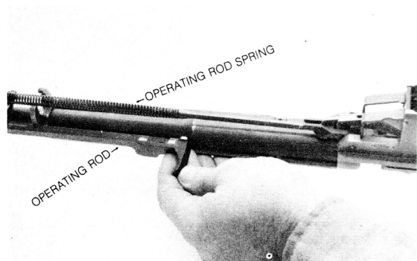
Figure 24. Removal / installation of operating rod assembly.
