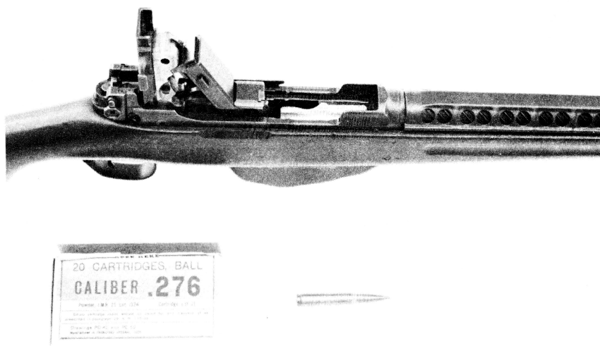
Figure 7. Close-up of Pedersen rifle - action open. Together with cartridge and box of ammunition. From the collection of Pierre Posse.
