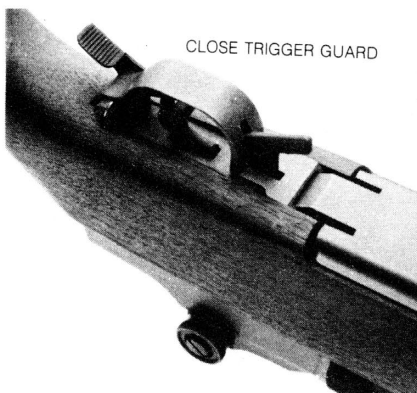
Figure 58. Installation of alternate winter trigger bit. Type T-36
