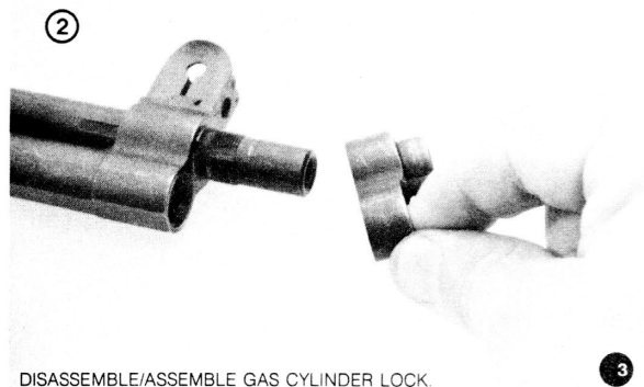
Figure 22. Disassembly / assembly of gas cylinder group (1 of 2).
