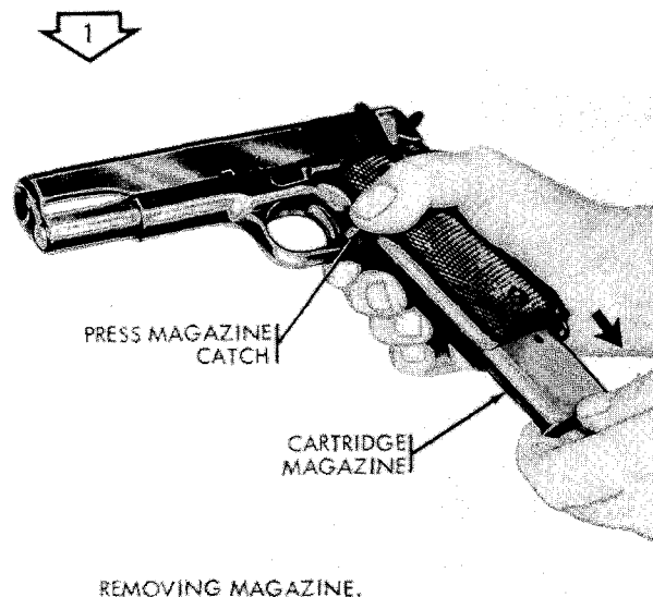
Figure 3-6. Operator's disassembly/assembly of Calilber .45 Automatic pistol, M1911A1. (1 of 3)
