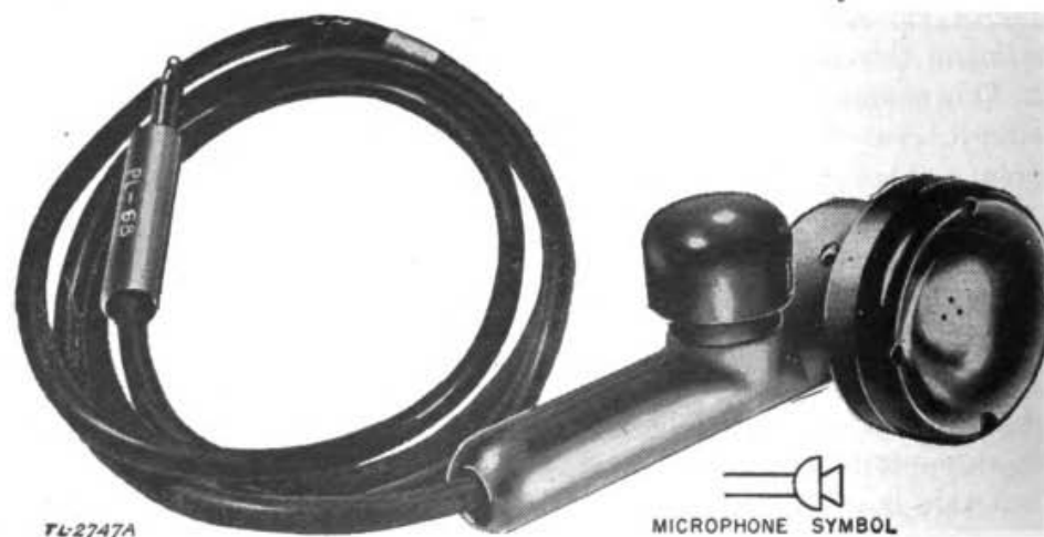
Figure 20. Carbon microphone T-17.
