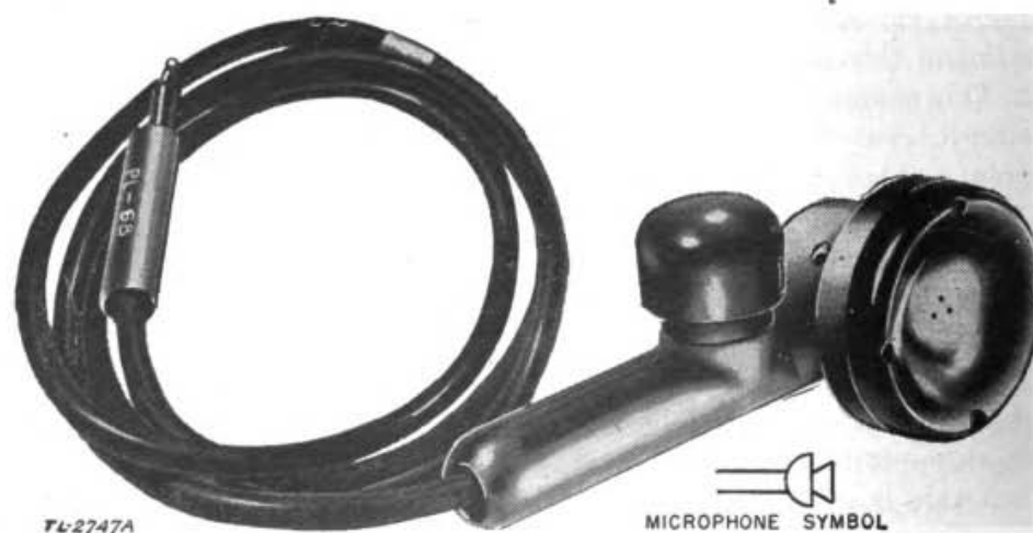
Figure 20. Carbon microphone T-17.
