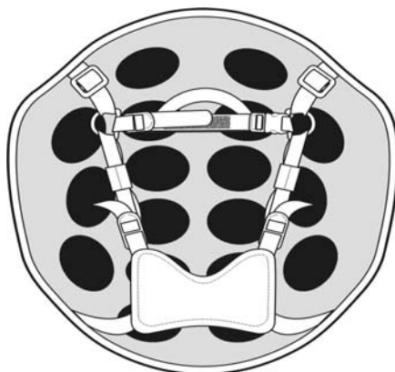
Figure 6. Chin Strap Retention System Orientation (Gentex X).
