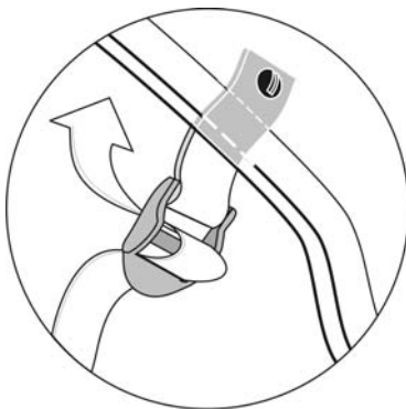
Figure 10. Routing of Chin Strap Webbing through Buckle (Gentex H).
