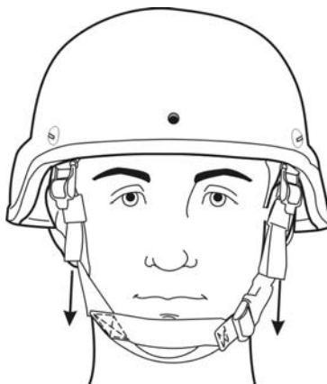
Figure 4. Tighten Front Adjustment Straps (All Versions).
