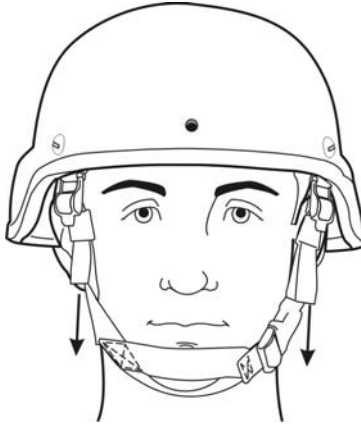
Figure 4. Tighten Front Adjustment Straps (All Versions).
