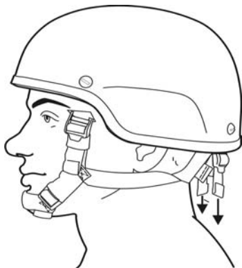
Figure 3. Tighten Rear Adjustment Straps (All Versions).
