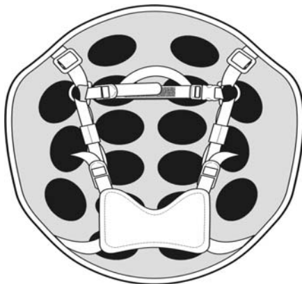
Figure 6. Chin Strap Retention System Orientation (Gentex X).
