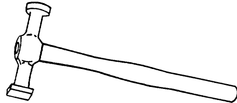
Figure 4-2. Body Hammer
