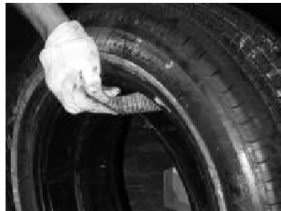
Figure 18. Pulling Strap Over Top of Runflat
