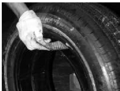
Figure 18. Pulling Strap Over Top of Runflat
