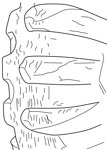
Figure 17. Oxidation of the Tire Tread
