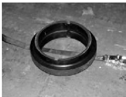
Figure 29. Preparing to Compress Runflat
