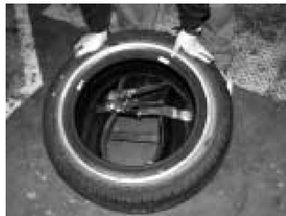
Figure 34. Runflat on Floor with Ratchet Handle Up
