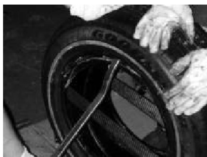
Figure 22. Inserting the Tire Iron
