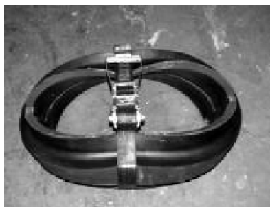
Figure 31. Compressing the Runflat
