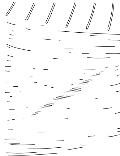
TEAR IN BEAD AREA
