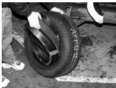
Figure 32. Inserting the Runflat into Tire Cavity
