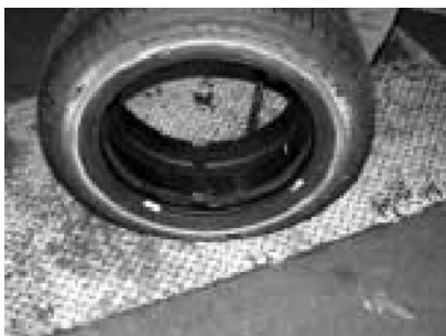
Figure 37. Aligning Runflat with Tire Beads
