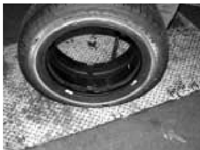
Figure 37. Aligning Runflat with Tire Beads
