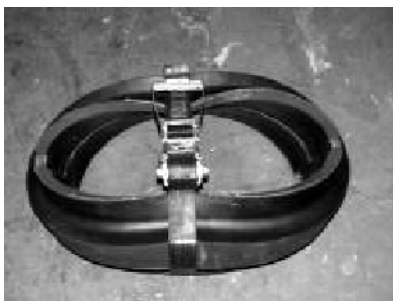
Figure 26. Runflat in Compressed State
