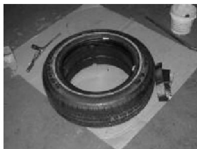
Figure 17. Preparing to Remove Runflat
