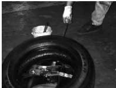
Figure 25. Extracting the Runflat From the Tire
