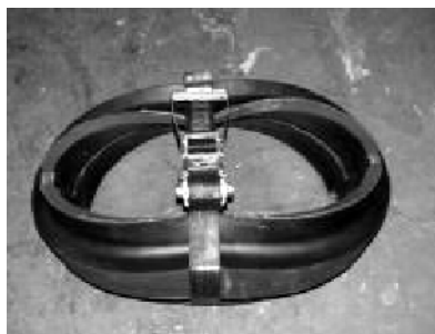
Figure 26. Runflat in Compressed State
