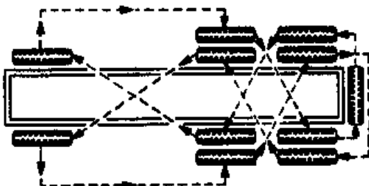
6x6 (DT). BIAS, BIAS BELTED, AND RADIAL TIRES
