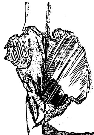
TREAD SEPARATION FROM CASING
