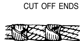
6 BEND TWISTED PORTION DOWN AGAINST ROPE
