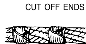
6 BEND TWISTED PORTION DOWN AGAINST ROPE
