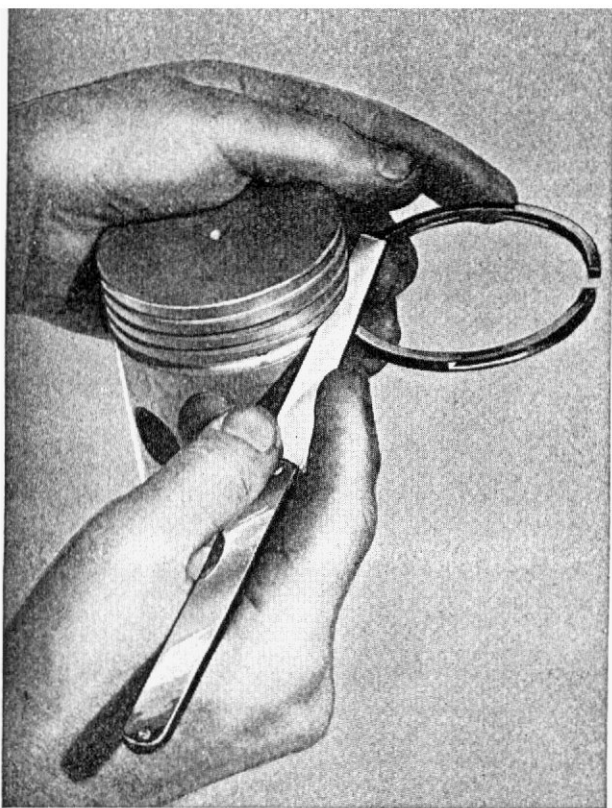
FIG. 27—OIL RING FITTING
