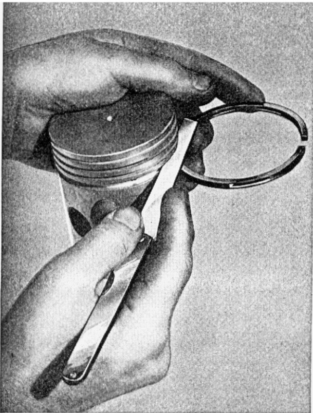
FIG. 27—OIL RING FITTING
