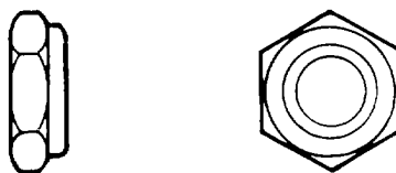
Figure 2-14. Self-Locking Thin Nut
