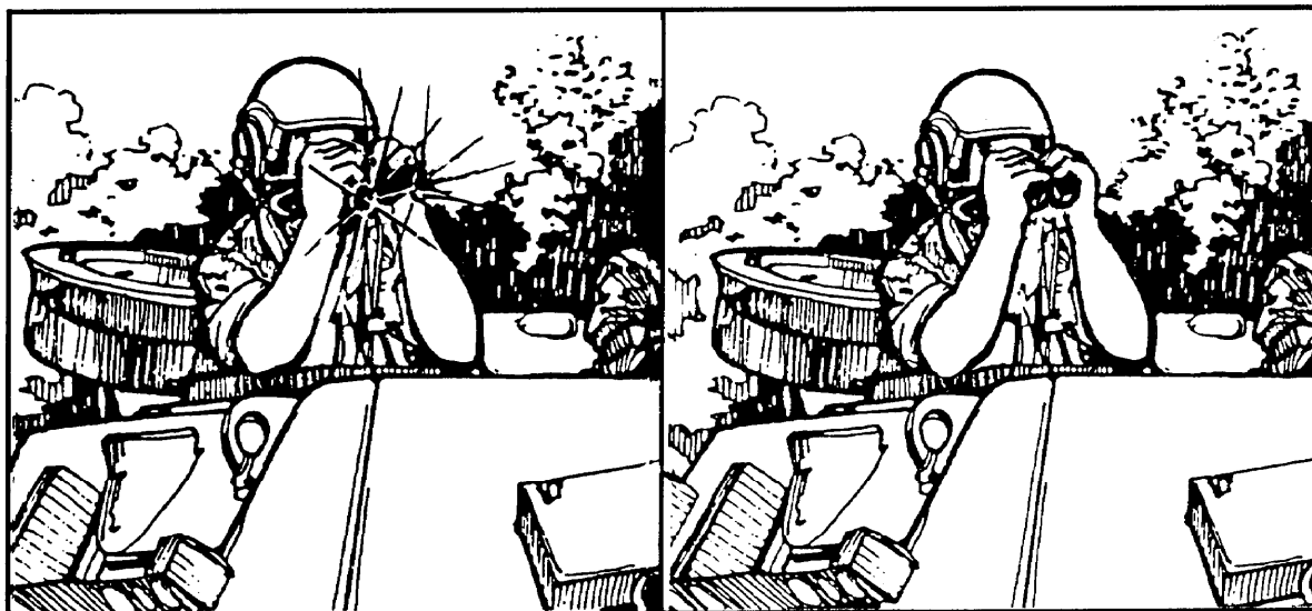
Figure E-1. Shade optics to prevent shine.
