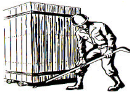
Figure 4-20. Use of wedge point bar and rollers
