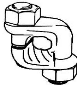
Figure 6-26. Improved type of wire rope clip
