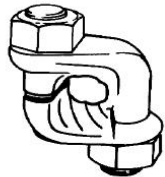
Figure 6-26. Improved type of wire rope clip
