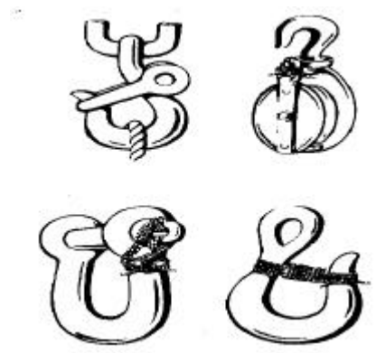
Figure 3-4. Mousing hooks
