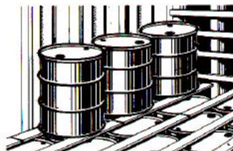
Figure 8-7. Use of dunnage in stowing drums
