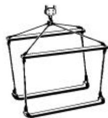
Figure 4-16. Pallet bridle spreaders
