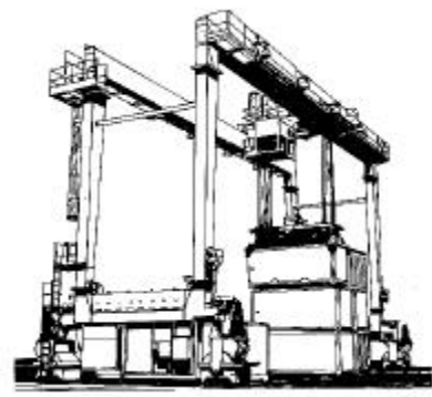
Figure 13-1. Straddle cranes in a piggyback operation
