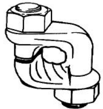
Figure 6-26. Improved type of wire rope clip
