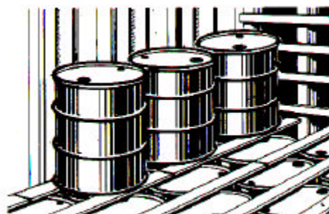
Figure 8-7. Use of dunnage in stowing drums
