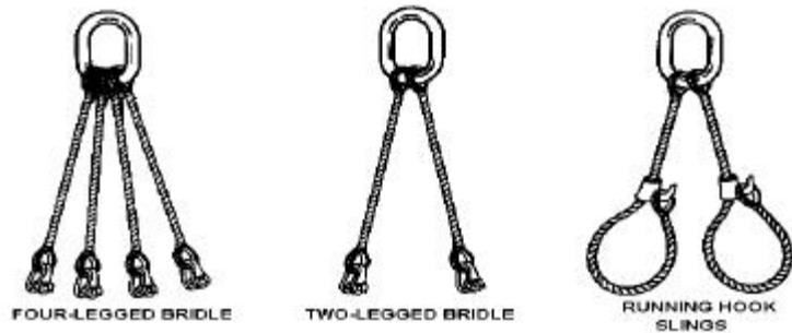
Figure 4-5. Combination slings
