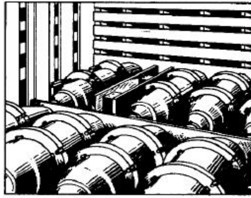
Figure 9-11. Dunnage used to separate bombs
