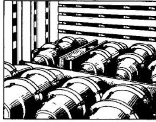
Figure 9-11. Dunnage used to separate bombs
