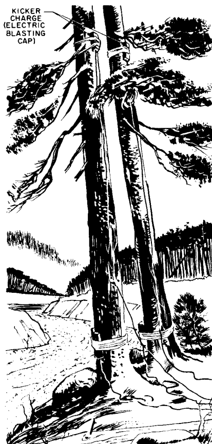
Figure 94. External timber-cutting charge.
